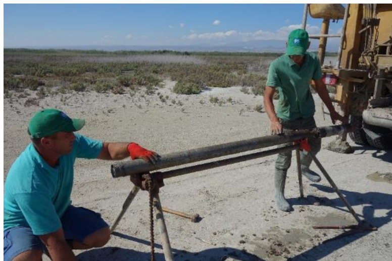
Figure 3 – Drilling (on the left) and extraction of the sedimentary core (on the right)
