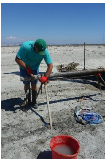
Figure 4 – Extraction of the sedimentary core sequence (Core Ak-1: -1.20 to -2.40 below the topographic level)
