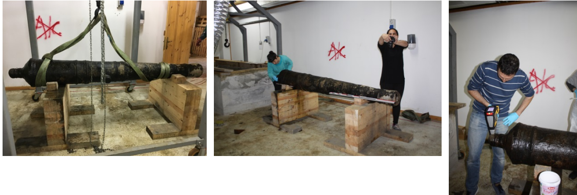
The cannon as lifted from its desalination tank during the replacement of the electrolyte which offered the opportunity to record it and carry out XRF analysis
