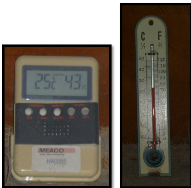
Figs. 6-7: Digital thermohygrometer (left) and thermometer (right) displaying the relative humidity and temperature of the Ship Gallery. These devices are aged and new equipment is needed.
