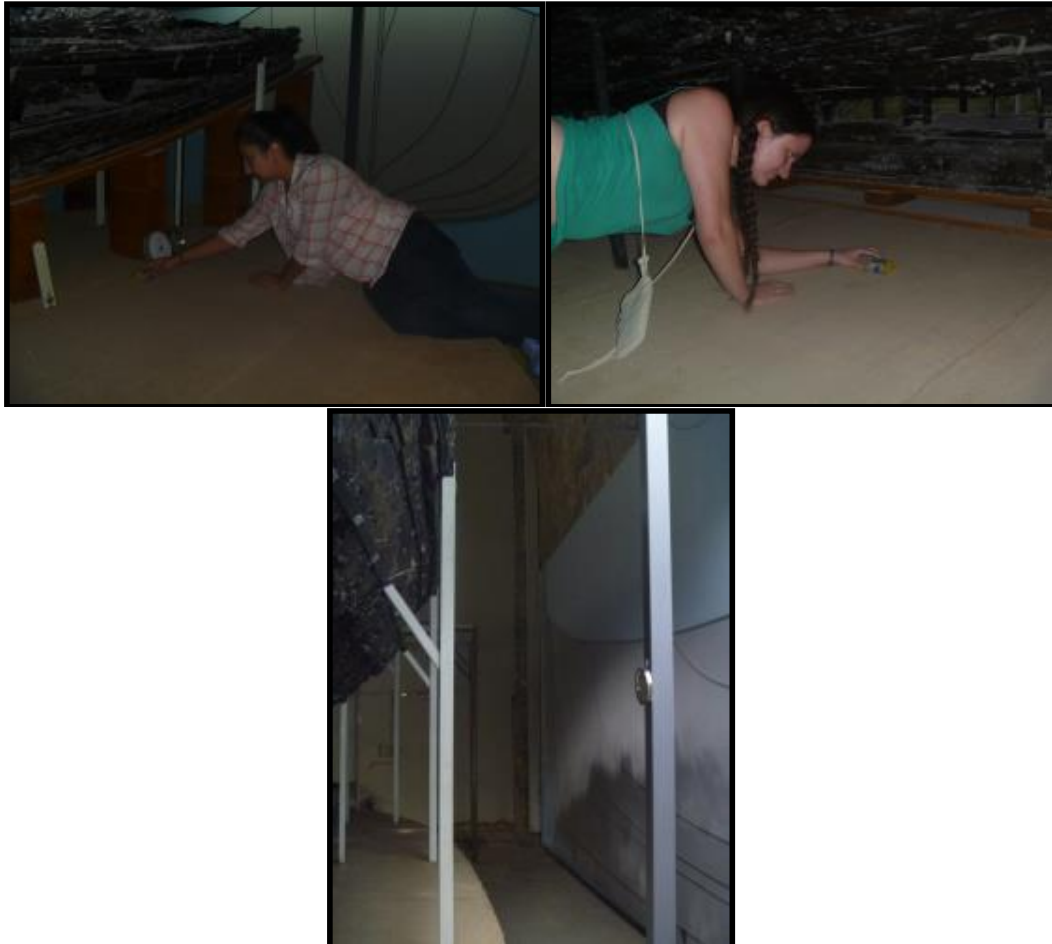
Figs 4-6: Photographs of conservators Cassy Cutulle (left) and Veronica Ford (right) installing Tiny Tag data loggers underneath the Ship Hull, along with the location of a newly installed analog thermohygrometer (below) in the Ship Gallery (Photographs courtesy of Veronica Ford, Cassy Cutulle 2016).
