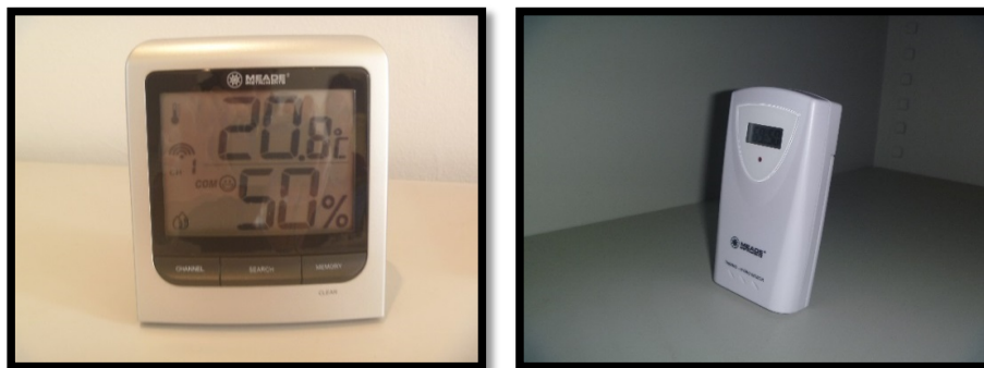
Figs. 5-6: Photographs of the electronic thermohygrometer used to track the temperature and relative humidity in the Conservation Laboratory in Nicosia. The left photograph displays a picture of the electronic temperature and relative humidity display while the right shows the sensor in the object storage cupboard. Photographs courtesy of Cassy Cutulle, 2016.
