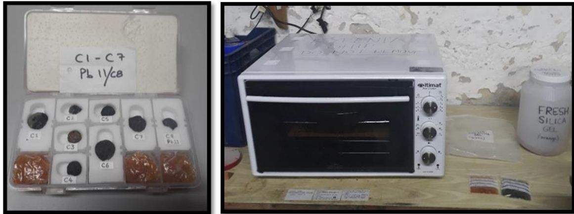
Figs.1-2: Photographs of the replaced silica gel in the coins storage (left) and the oven required for dehydrating green silica gel (right) (Photographs courtesy of Veronica Ford, 2017).
