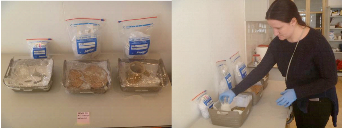
Fig. 7: (Left) Photograph of the first three ceramic objects for desalination in a high humidity atmosphere to prime the ceramic prior to desalination soaking. (Right) Photograph of Veronica Ford placing a beaker of tap water with cotton wool in the basin to create the humid atmosphere. Photograph courtesy of Cassy Cutulle, 2016.
