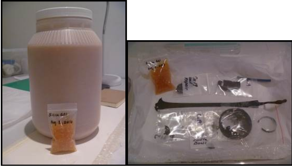
Figs. 4-5: Photographs of the silica gel used to control the relative humidity in the boxes storing metal objects.
