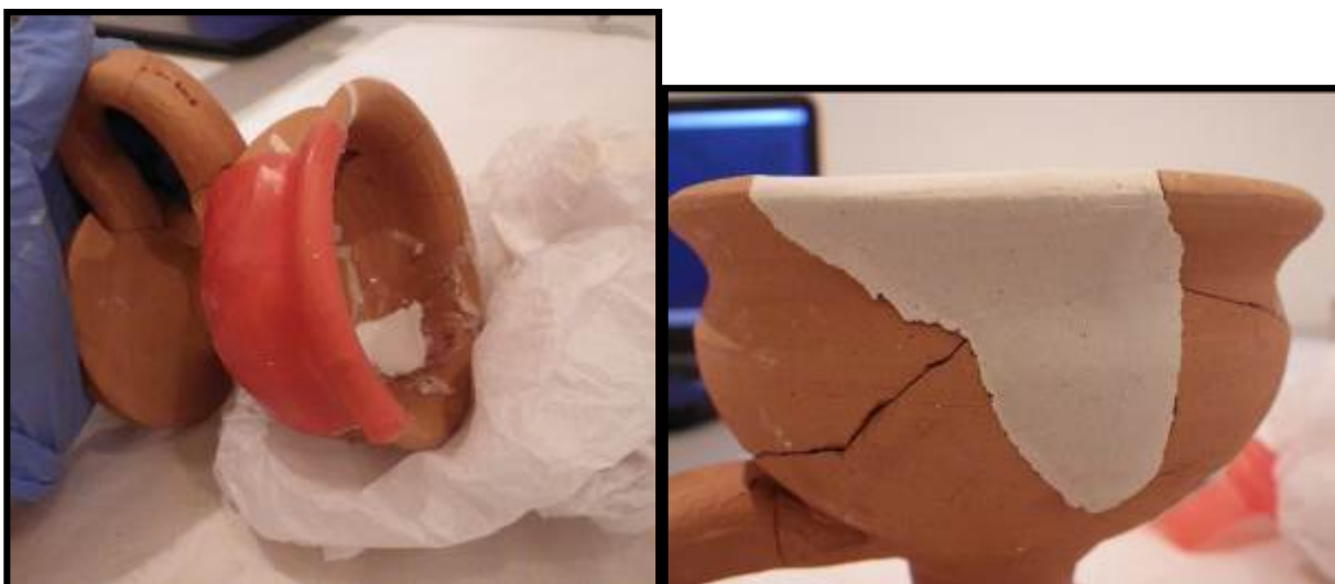
Fig. 12: Photographs of the wax mold with fill in place, drying (left) and the results of the dried fill (right) (Photographs courtesy of Veronica Ford, 2016).
