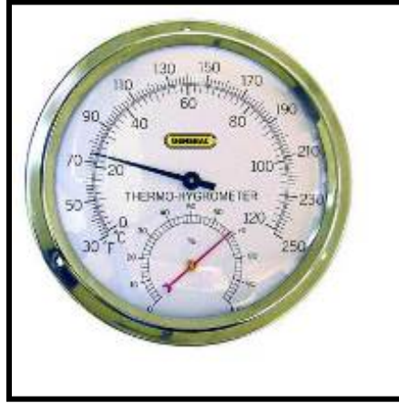
Figs.5-6: (Left) Image of an electronic Tiny Tag relative humidity/temperature data logging device and (right) image of an analog thermohygrometer, which shows the relative humidity and temperature in real-time. (Images courtesy of: http://www.gemindataloggers.com/data-loggers/tinytag-ultra-2 and http://www.homedepot.com/p/General-Tools-Indoor-Analog-Thermo-Hygrometer-with-5-in-Dial-and-Stainless-Steel-Case-A600FC/202735076 , 2016)
