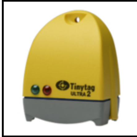
Figs.5-6: (Left) Image of an electronic Tiny Tag relative humidity/temperature data logging device and (right) image of an analog thermohygrometer, which shows the relative humidity and temperature in real-time. (Images courtesy of: http://www.gemindataloggers.com/data-loggers/tinytag-ultra-2 and http://www.homedepot.com/p/General-Tools-Indoor-Analog-Thermo-Hygrometer-with-5-in-Dial-and-Stainless-Steel-Case-A600FC/202735076 , 2016)
