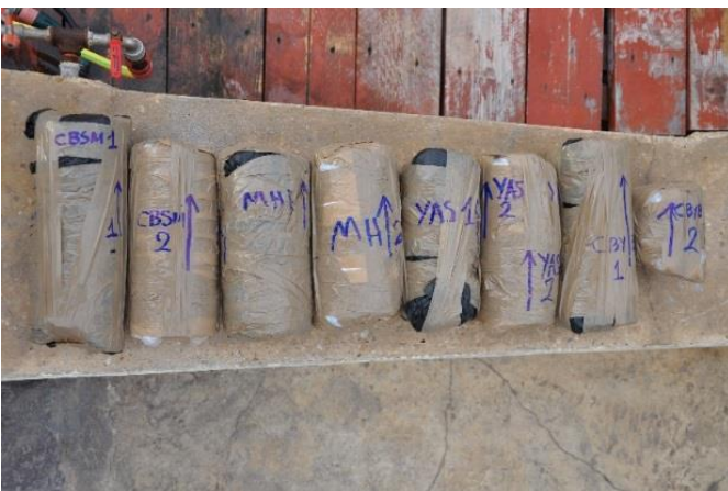
Figure 6. Rock samples (Turoneun limestone covered by Dendropoma Petraeum ) extracted from uplifted platforms for dating by Optically Stimulated Luminescence (OSL) and Carbon 14 (C14); (©Byblos & the Sea, 2016, G. Papatheodorou; Photo M. Francis-Allouche).
