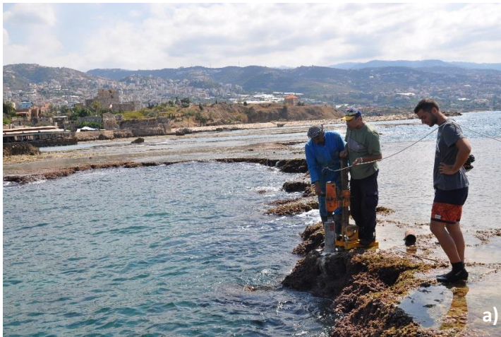
Figure 5. The sampling procedure on geological platforms (a): the wet diamond core drill (b) and the hammer & chisel technique (c); Photo M. Francis-Allouche).
