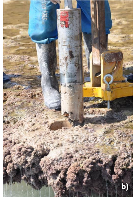
Figure 5. The sampling procedure on geological platforms (a): the wet diamond core drill (b) and the hammer & chisel technique (c); Photo M. Francis-Allouche).
