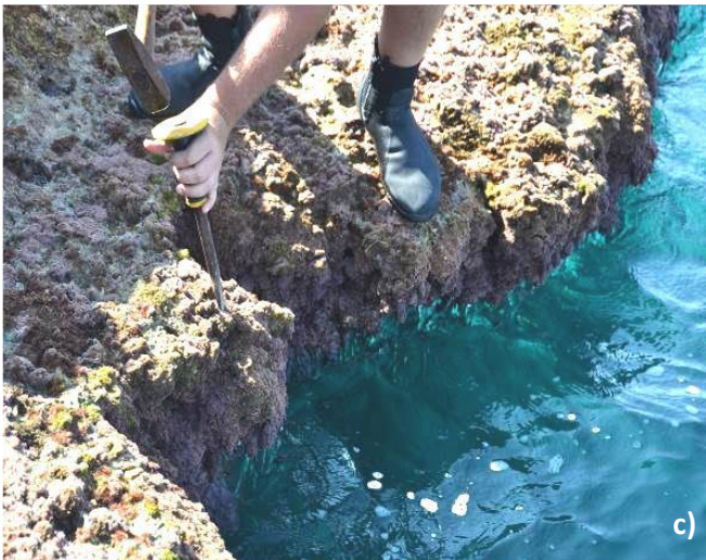
Figure 5. The sampling procedure on geological platforms (a): the wet diamond core drill (b) and the hammer & chisel technique (c); Photo M. Francis-Allouche).
