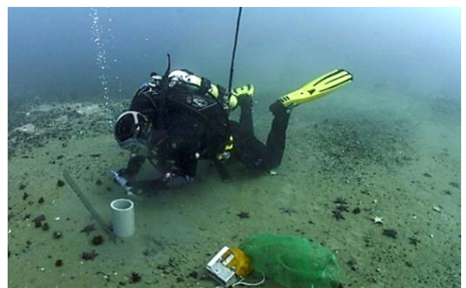
Figure 5. Map of nearshore maritime area of Byblos and diver in the Bay of Jouret Osman using PVC tube to collect short sediment cores (marked with blue star); (©Byblos & the Sea, 2016, G. Papatheodorou).
