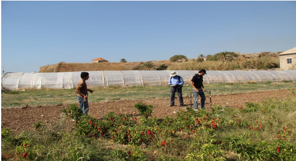
Figure 2. Electrical resistivity survey at the southern foot of the archaeological tells of Byblos, on the Armenian Orphanage lot; Geophysicist, Tomasz Herbich, taking electrical resistivity profiling measurements.
