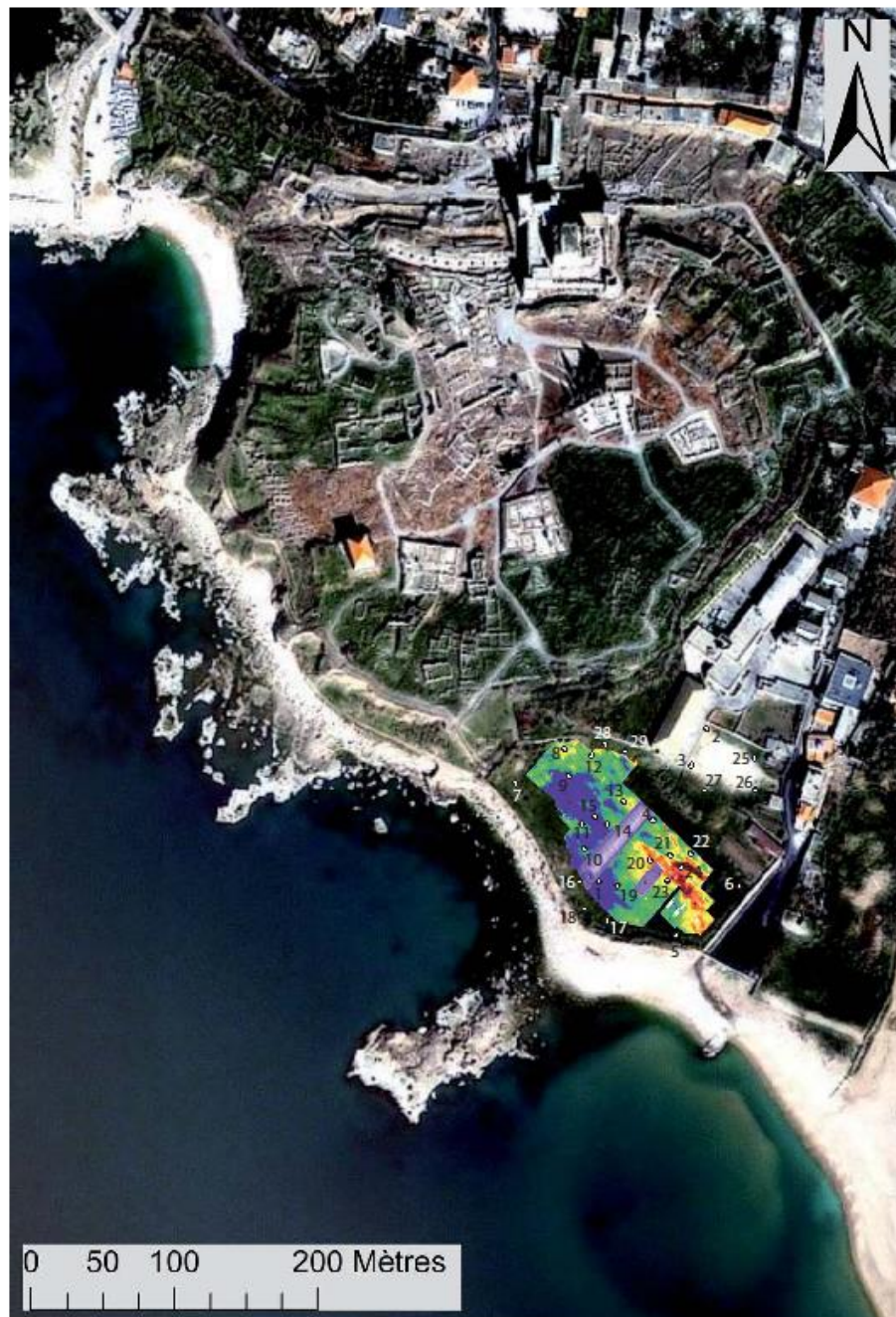
Figure 4. Geophysical 2D image of the underground in the lower Armenian Orphanage lot, showing the buried basin and drilling location of 29 boreholes to verify its existence (mission 3).
