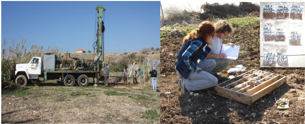
Figure 2. An example (left) of the 29 auger coring drills performed at 6m depth; sediment specialist N. Carayon (right) analyzing sediments extracted from coring; sample sediments (far right) sent for analyses & dating to laboratory (©Byblos & the Sea, 2014, Martine Francis-Allouche and Nicolas Grimal).
