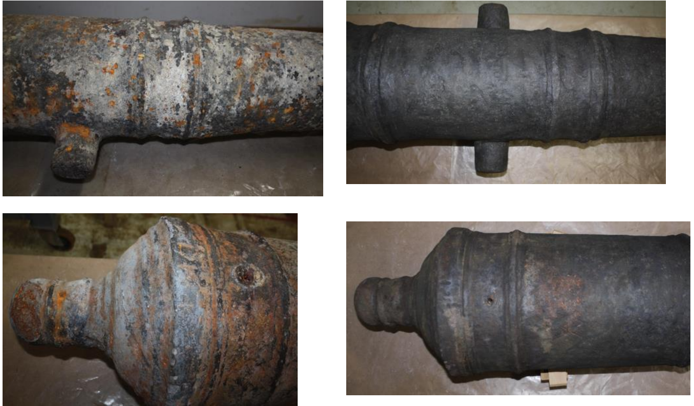
Fig. 6 : Iron cannon (ESEA 62-14 ) before and after cleaning.
